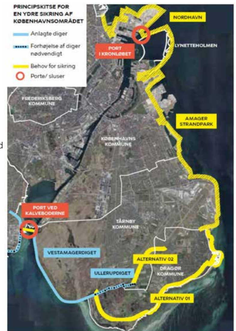
Figure 21. Copenhagen. Planning for levees (“diger”). Blue have already been put in place, yellow are to come.
